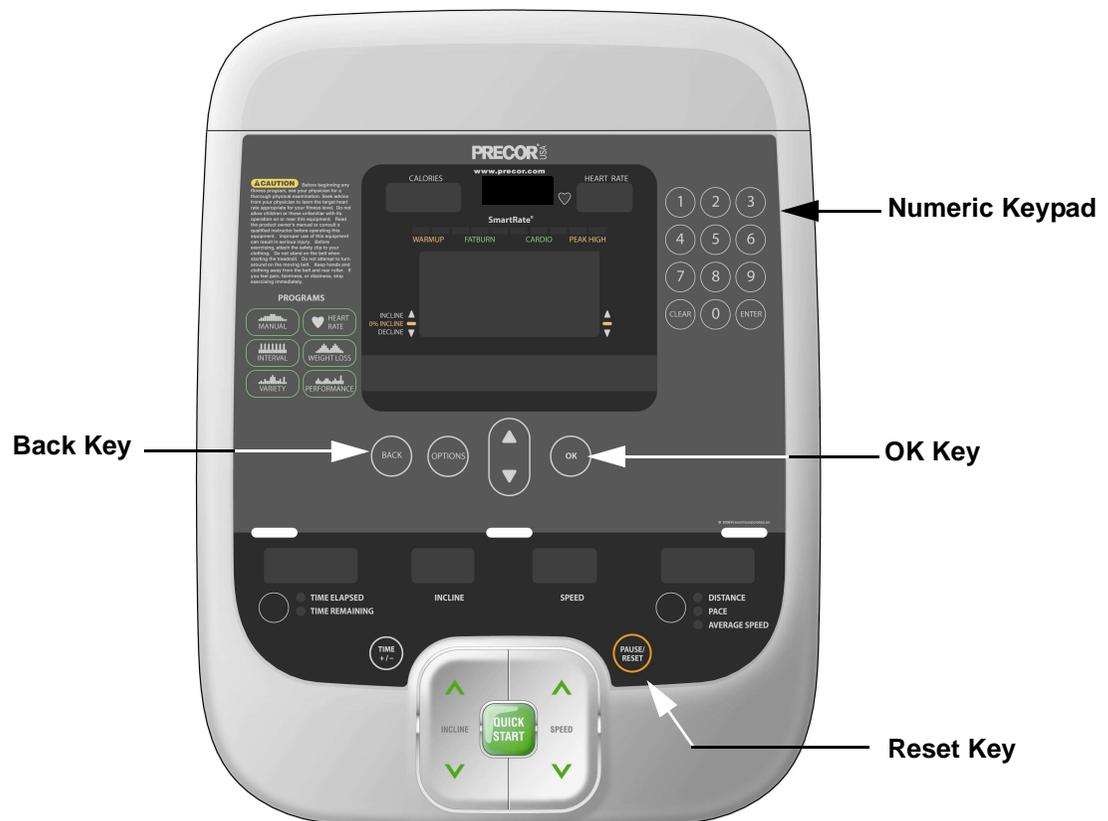
4. Press the **OK** key, the upper most group of LED's will illuminate on the display. Check the display to ensure that all LED segments are illuminated.
